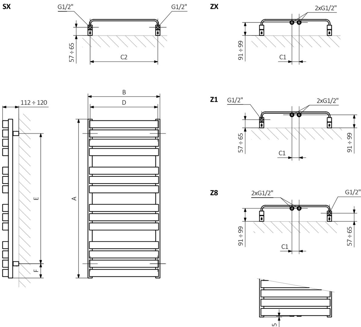
A – Height B – Width C1-C5 – Distance between pipe centres D – Horizontal distance between mounting bracket centres
