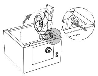
Lift the motor up by holding the motor bracket's handle, keep fingers away from the back of the hinge. Make sure that the motor bracket attach to the lock to prevent the motor from falling down during maintenance. After maintenance, release the lock, using the handle to bring the motor down. Fasten the motor bracket with the screws.
