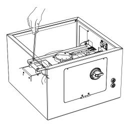
Unscrew the motor bracket's two screws.
