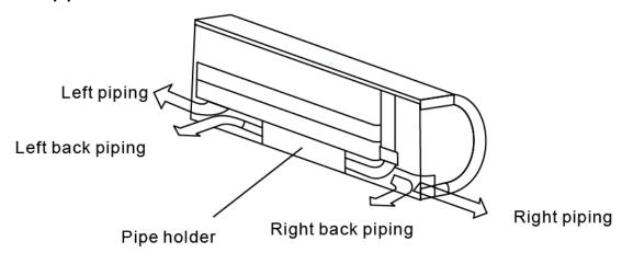
For the left-hand and rear-left-hand piping, install the piping as shown. Bend the connective pipe to be laid at 43mm height or less from the wall.
