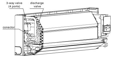
■ At the first debugging, completely expel air from coils via expelling valve.
