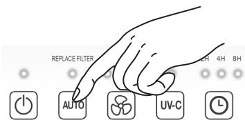
6. Insert the mains plug into the socket. Ensure that the cable does not pose a trip hazard. Press and hold the AUTO button (**AUTO**) for five seconds. The operating hours counter now resets to 0.
