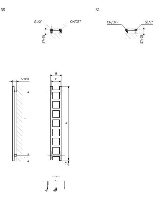
A - Height B - Width C1-C5 - Distance between pipe centres D - Horizontal distance between mounting bracket centres E - Vertical distance between mounting brackets F - Distance between a mounting bracket and the bottom of the radiator
