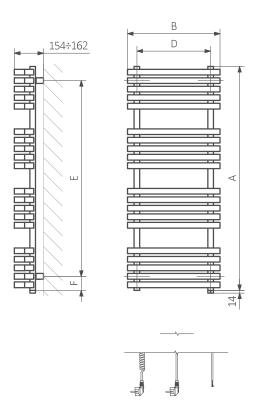
A - Height B - Width C1-C5 - Distance between pipe centres D - Horizontal distance between mounting bracket centres E - Vertical distance between mounting brackets F - Distance between a mounting bracket and the bottom of the radiator
