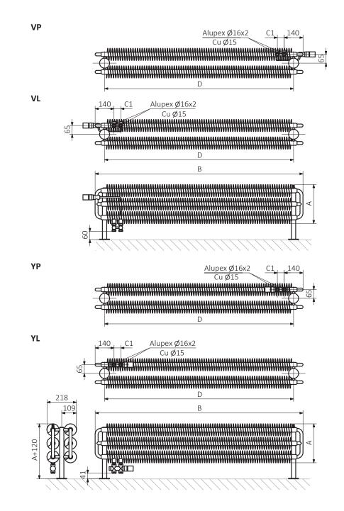
$\begin{array}{lll} A - \mbox{Height} & B - \mbox{Width} & \mbox{C1-C5} - \mbox{Distance between pipe centres} & \mbox{D} - \mbox{Horizontal distance between mounting bracket centres} \\ E - \mbox{Vertical distance between mounting brackets} & \mbox{F} - \mbox{Distance between a mounting bracket and the bottom of the radiator} \\ \end{array}$
