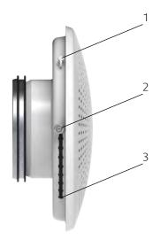
The diffuser is equipped by an adjustable blind that changes the effective air flow aperture and so tunes the air flow volume. The mechanism is movable from outside by a miniature knob. The movement has 9 fixed positions. For adjustment only these positions provide desired noise parameters. The intermediate positions shall be avoided.
