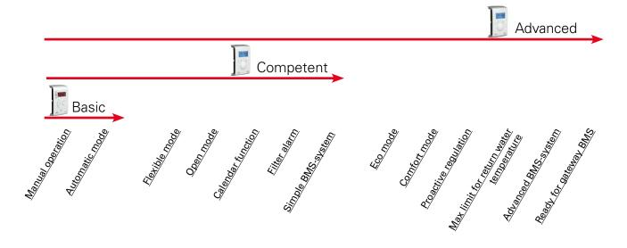
This air curtain is supplied with an intregrated PC board SIRe. There are three different levels with different functionality to choose from, Basic, Competent or Advanced.
