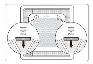
3 Hang the panel on the 2 hooks on the both sides of the indoor unit firmly so that the panel not to fall out.
